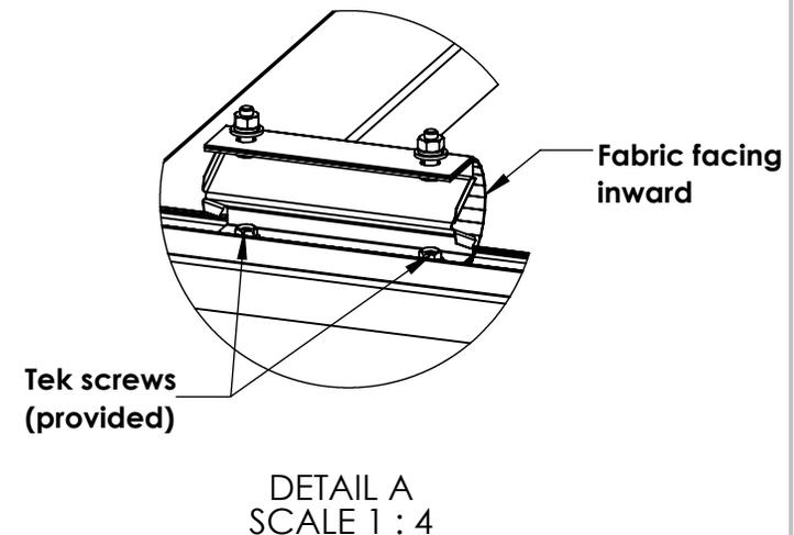
**STEP 4:** Set the top rails down onto the springs of each corresponding bottom rail. Inset the bolts up through the restraints and into the pre-drilled top rail. Secure with flat washer, lock washer and nut.
