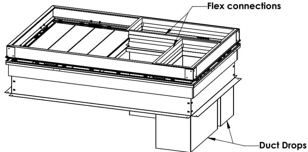
**STEP 6:** Install all duct supports provided with isolation rail using 14 x 1" Tek screws. locations and dimensions will be marked on submittal drawing.
