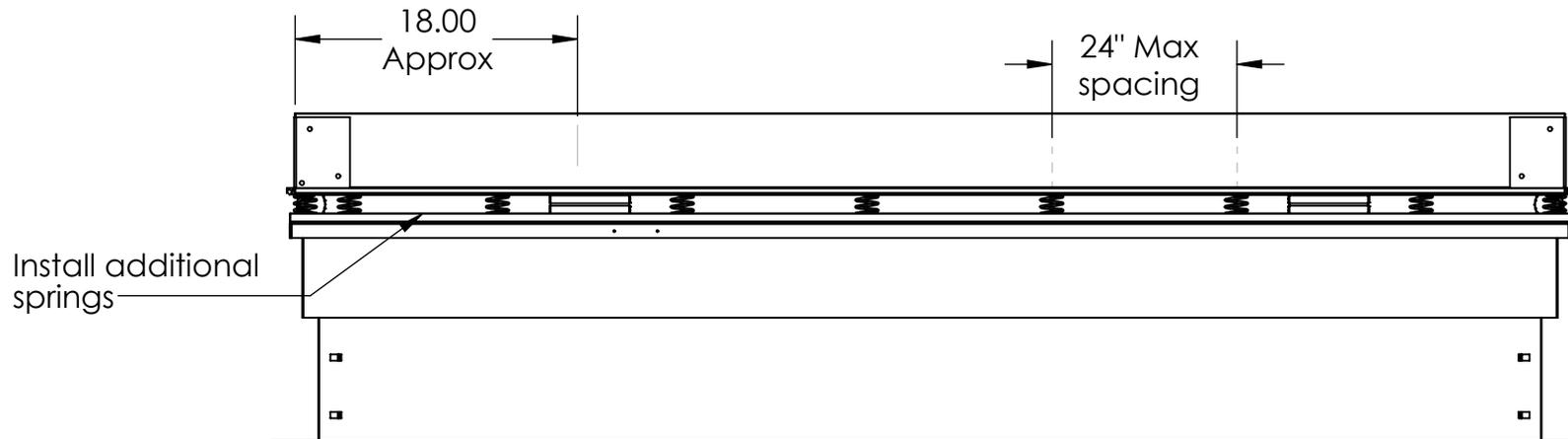
4. If unit leveling is required after crane has left, a bottle jack may be used raise the corners of the unit to install/remove springs.
