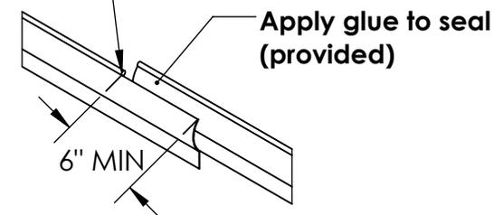
Once the weathersel is fully wrapped around the perimeter, overlap the cut end and use glue to seal. Additional trimming may be necessary for proper fitment.
