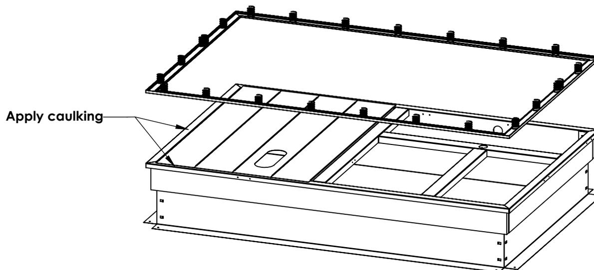
**STEP 3:** Install wind restraints in locations previously removed from the bottom rail. Use the (2) 1" long tek screws (provided) to attach restraint to curb through bottom rail and into top curb flange.
